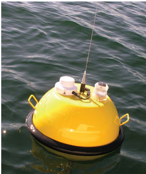
Figure 2-2: The TRIAXYS™ Mini directional Wave Buoy
