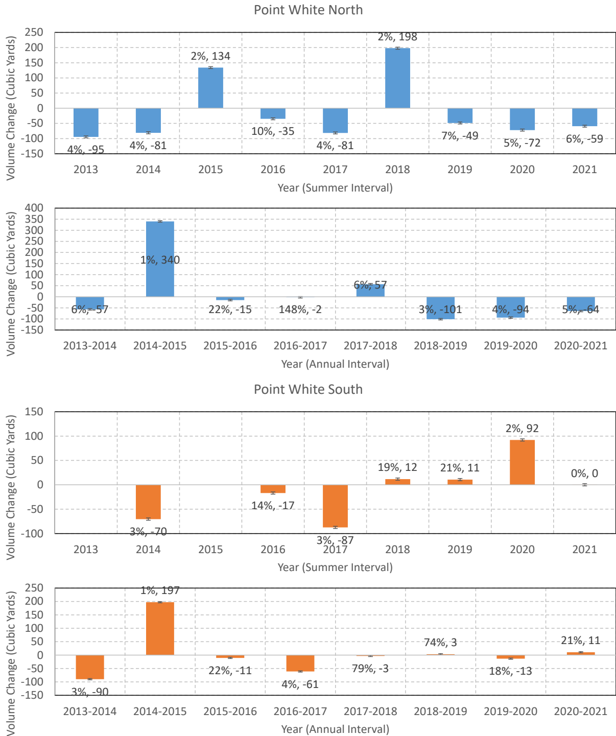
Figure 4. Volume change (cubic yards) in calculation area at Point White South and North. The volume change and error as a percent of the total change are shown for each measurement.
